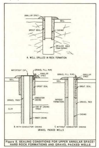
(4) <u>Wells situated in "hard" consolidated formations (crystalline or metamorphic rock)</u>. An oversized hole shall be drilled to the depth specified in Subsection (A), above, and the annular space filled with sealing material. If there is significant overburden, a conductor casing may
