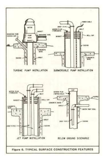
(1) Where the pump is installed direct over the casing, a watertight seal (gasket) shall be placed between the pump head and the pump base (slab), or a water-tight seal (gasket) shall be placed between the pump base and the rim of the casing, or a "well cap" shall be installed to close the annular opening
